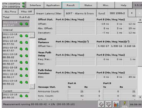
Fig. 15 Comprehensive IEEE 1588 v2 statistics on offset and offset variance, path delay variation, messages and clock state transitions.
