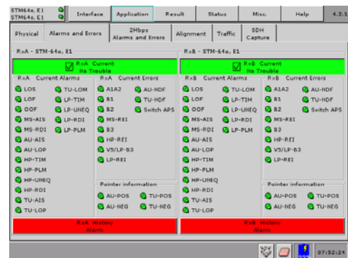
Fig. 26 The CMA 3000 gives you a quick overview of errors and alarms of both sides of the STM-64 line.
