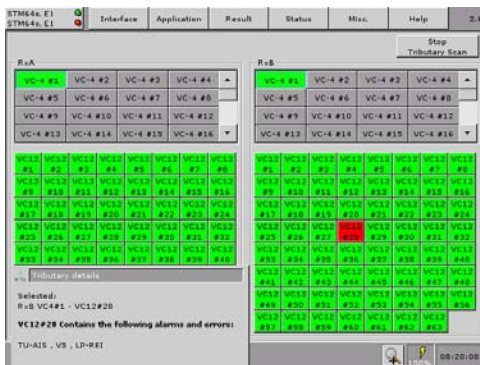
Fig. 27 The trouble scan feature gives you a quick overview of the tributaries of the monitored line.
