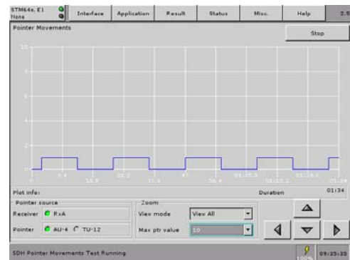
Fig. 28 The pointer graph allows a detailed analysis of pointer movements in the monitored STM-64 signal.
