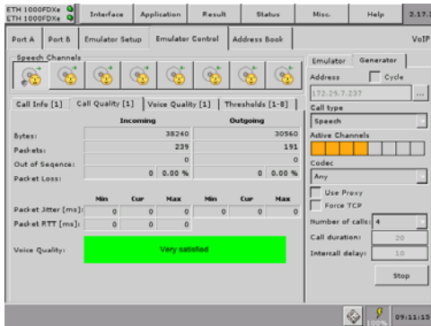
Fig. 20 A total of 8 VoIP calls can be generated through the CMA 3000's two Ethernet test ports. The voice quality evaluation is presented for one call if the Voice Quality Measurement option is installed.
